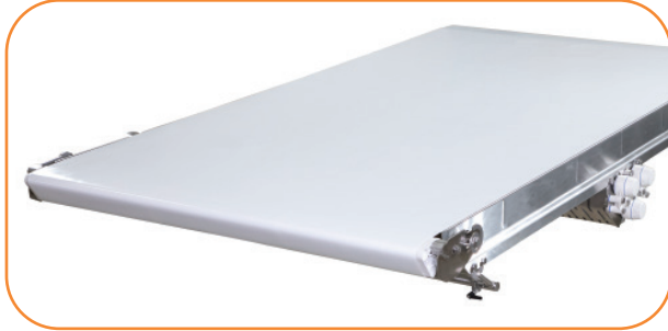
STANDARD FEATURE: V-Guided Belt Tracking
