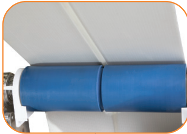
V-GUIDED BELTING FOR POSITIVE BELT TRACKING
